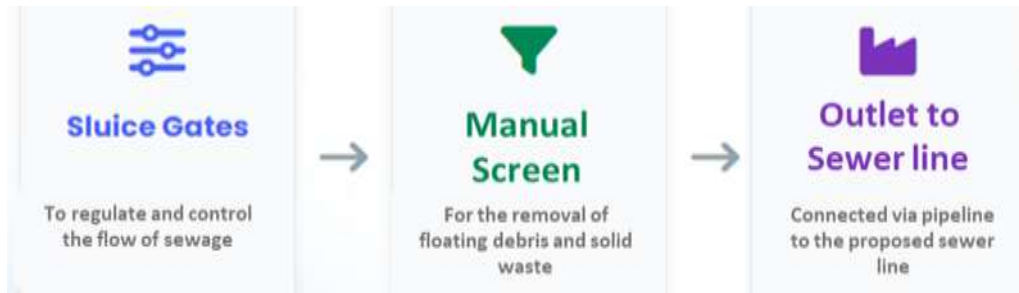
Figure 7-1: Flow arrangement of proposed I & D Structure
