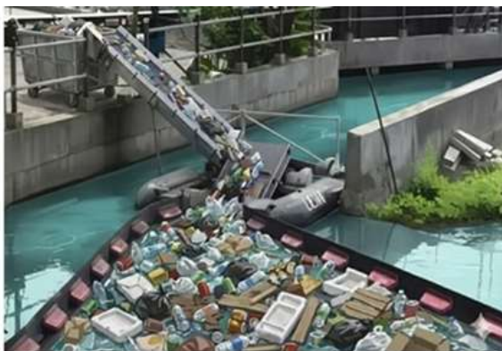
Picture 7-14: Proposed Riser-type Trash Trap systems (floating boom barrier, mechanical screen and belt conveyor)
