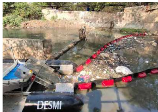
Picture 7-14: Proposed Riser-type Trash Trap systems (floating boom barrier, mechanical screen and belt conveyor)
